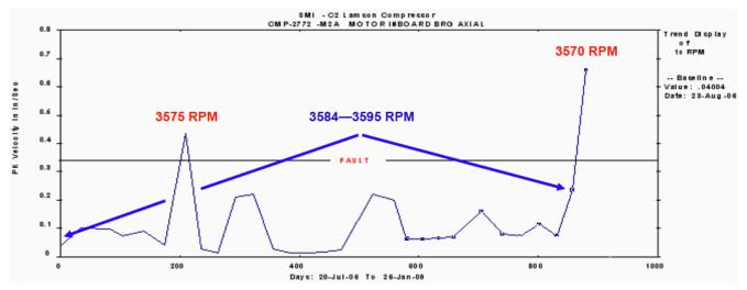
**Recommendatio**n: It was recommended that the #3 Lamson compressor's load be lessened to aid in decreasing the excessive vibration amplitudes.
